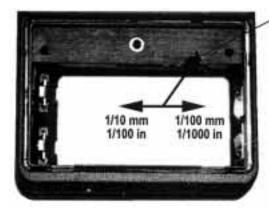
Here you will find the slide switch to alter the display resolution • Fit batteries again and close the battery compartment.
